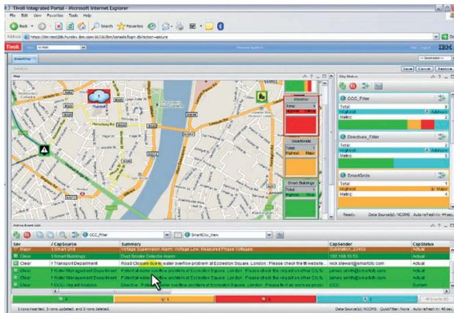
Tivoli Netcool/Impact automatically collects information across multiple support tools and data sources and displays that information in context in a single, integrated web view
